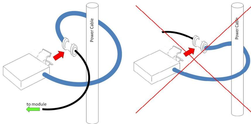
The sensor has to be properly aligned to the cable, as shown in the following figure.
